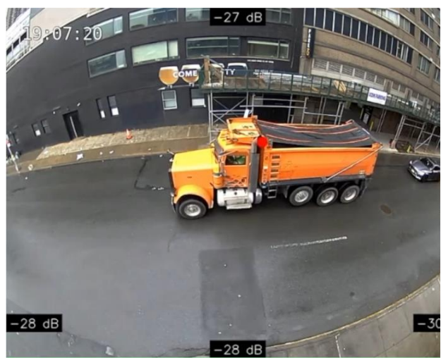
Figure 3-6: Acoustic Camera Imaging Example – Identifying a loud dump truck exhaust
