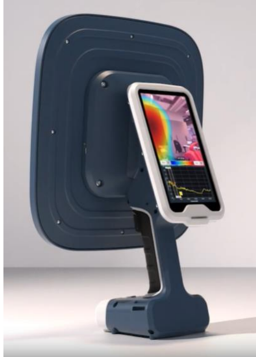
Figure 3-6: Acoustic Camera Imaging Example – Identifying a loud dump truck exhaust
