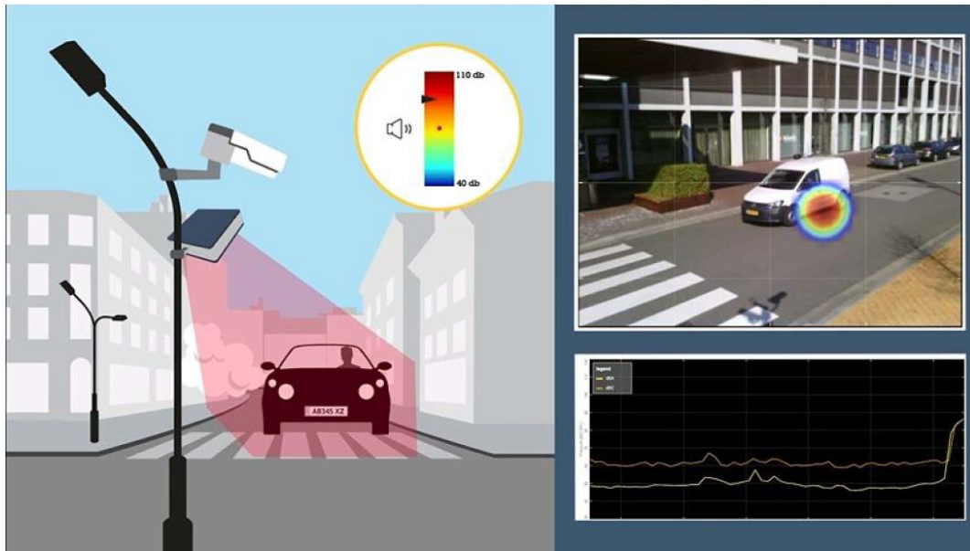
Figure 4-2: Example of a Fixed Acoustic Camera System
