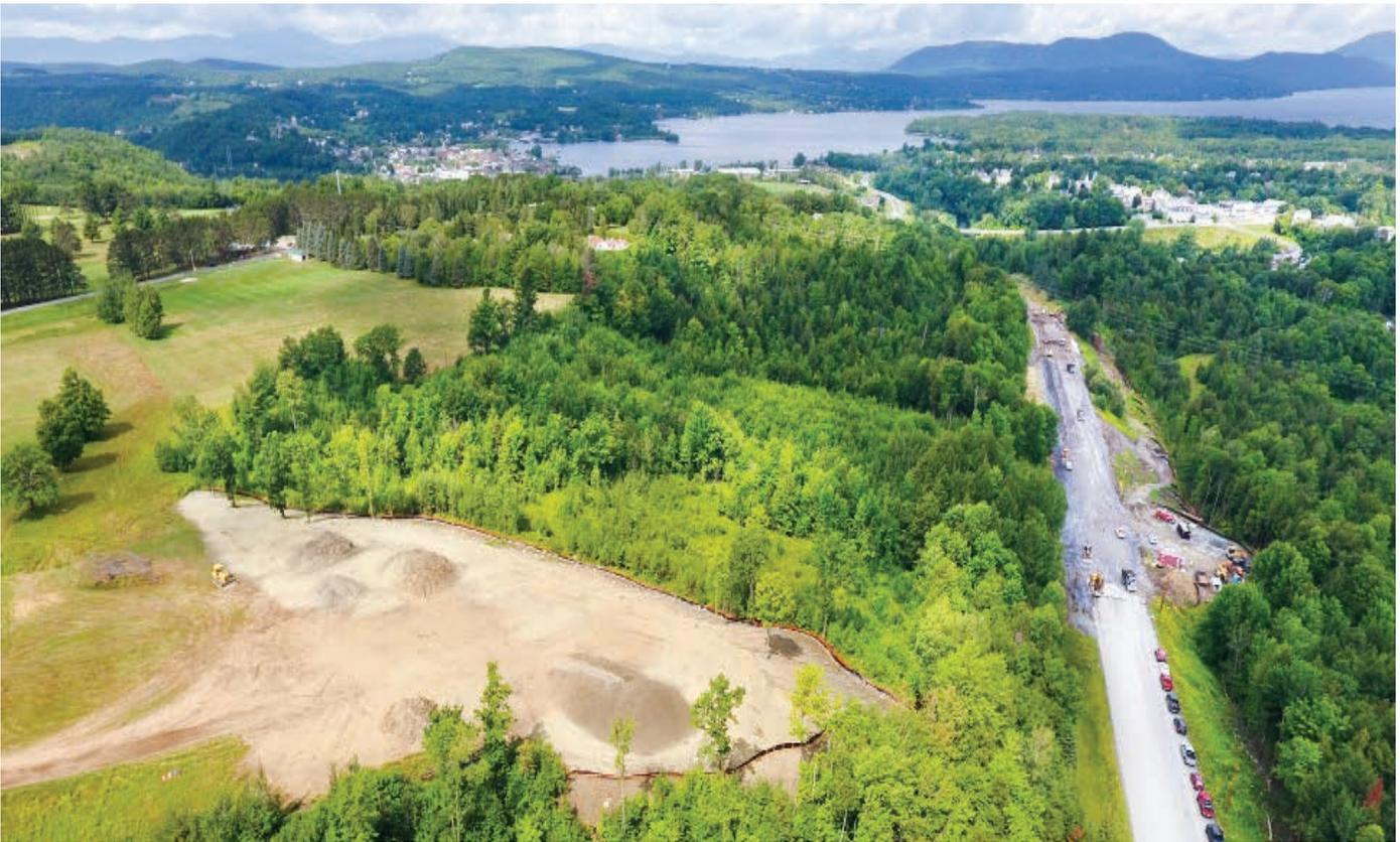
**NEWPORT CITY.** Remediating slope failures along VT-191 required full-depth reconstruction of the roadway, replacement of a failed culvert, and installation of three active wells to extract water from below the road surface.
