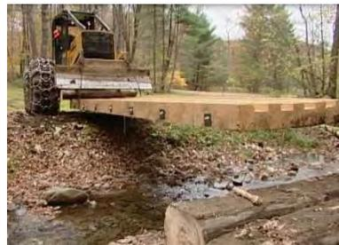
Portable skidder bridge in action, see Figure 16
