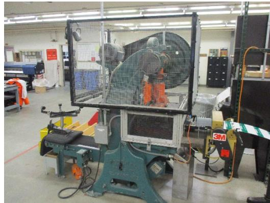
From there, the plates are now ready to be “gauged”. This is where VCI workers will stack pairs of plates into piles of 50 pairs in preparation to be pressed with digits/characters.
