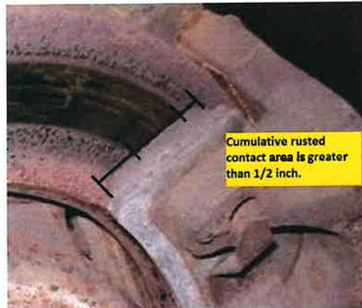
**Note:** Rust is defined as a condition of any swelling, delamination, or pitting.
