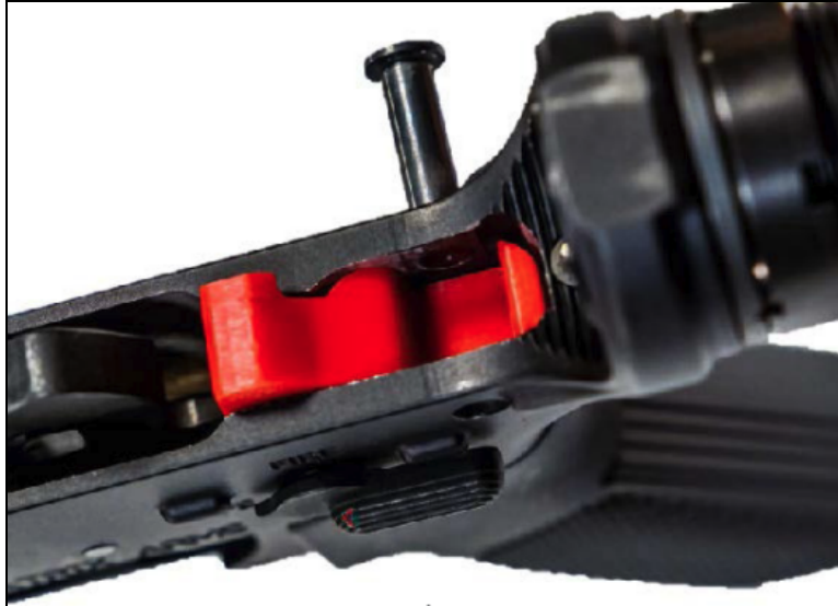
A red, 3D-printed auto sear is shown inside an AR-15.
