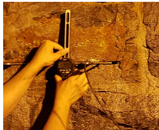
Image 10. Flat Jack Test. Stevens & Associates 07.17.2023
