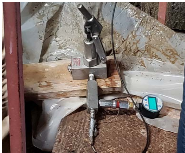
Image 14. Goodman Jack Test. Stevens & Associates 07.17.2023
