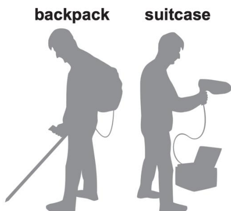
Figure 1. Examples of most common implementation of portable LIBS. Adapted from Rokovsky et al. 1 .
