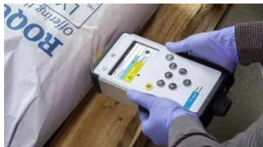
Figure 2. Example of a commercial handheld Raman system. Adapted from agilent.com.
