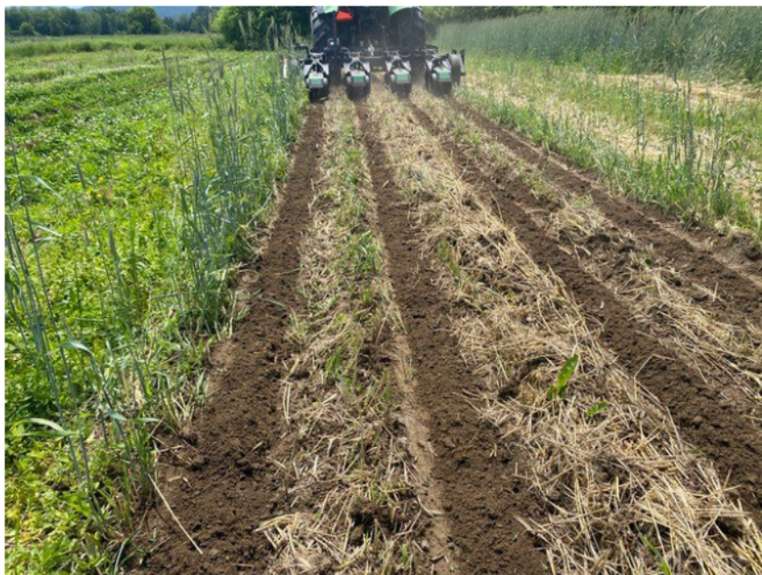
Figure 4. A CRWFA member utilizes the strip tillage conservation equipment unit to prepare a field for planting with reduced tillage techniques.
