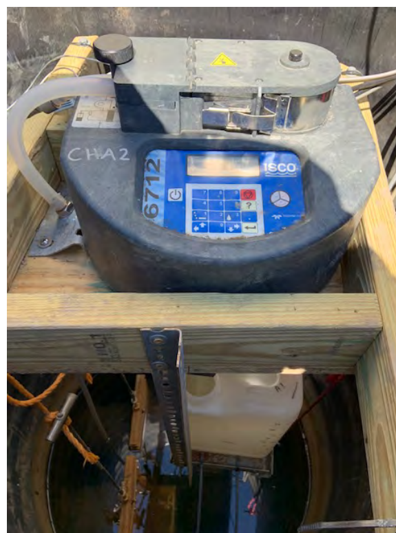
Figure 15. Custom autosampler rack in monitoring manhole
