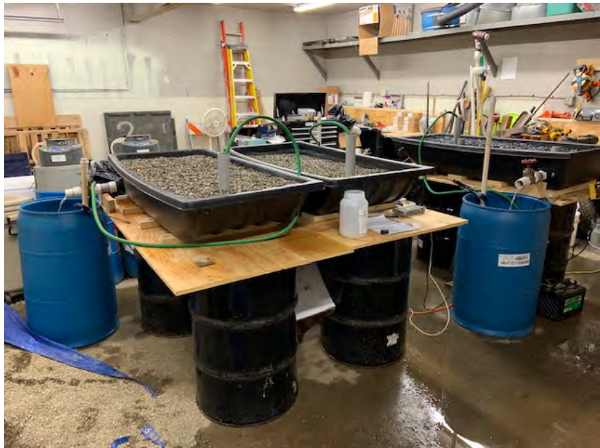
Figure 10. Three filter sleds recirculating P solution
