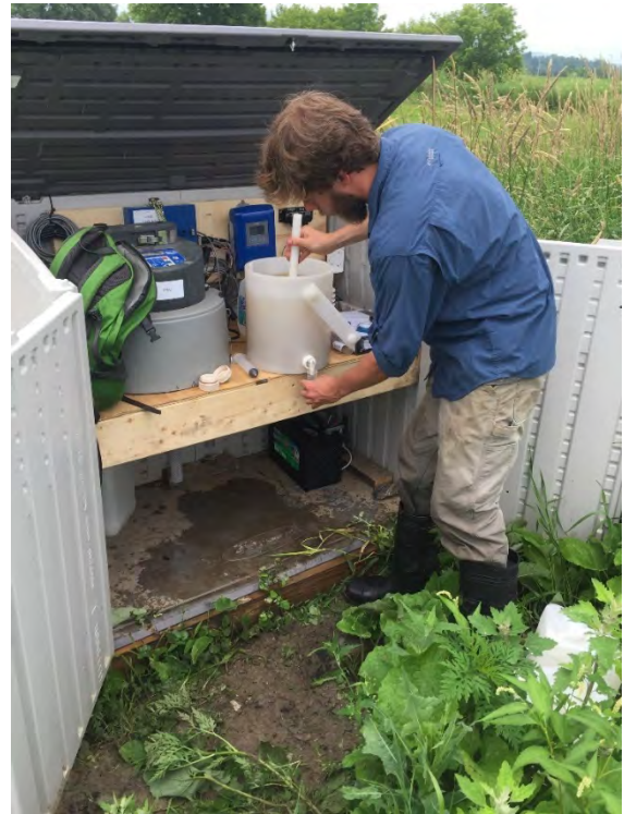
Figure 9. Processing a composite water sample
