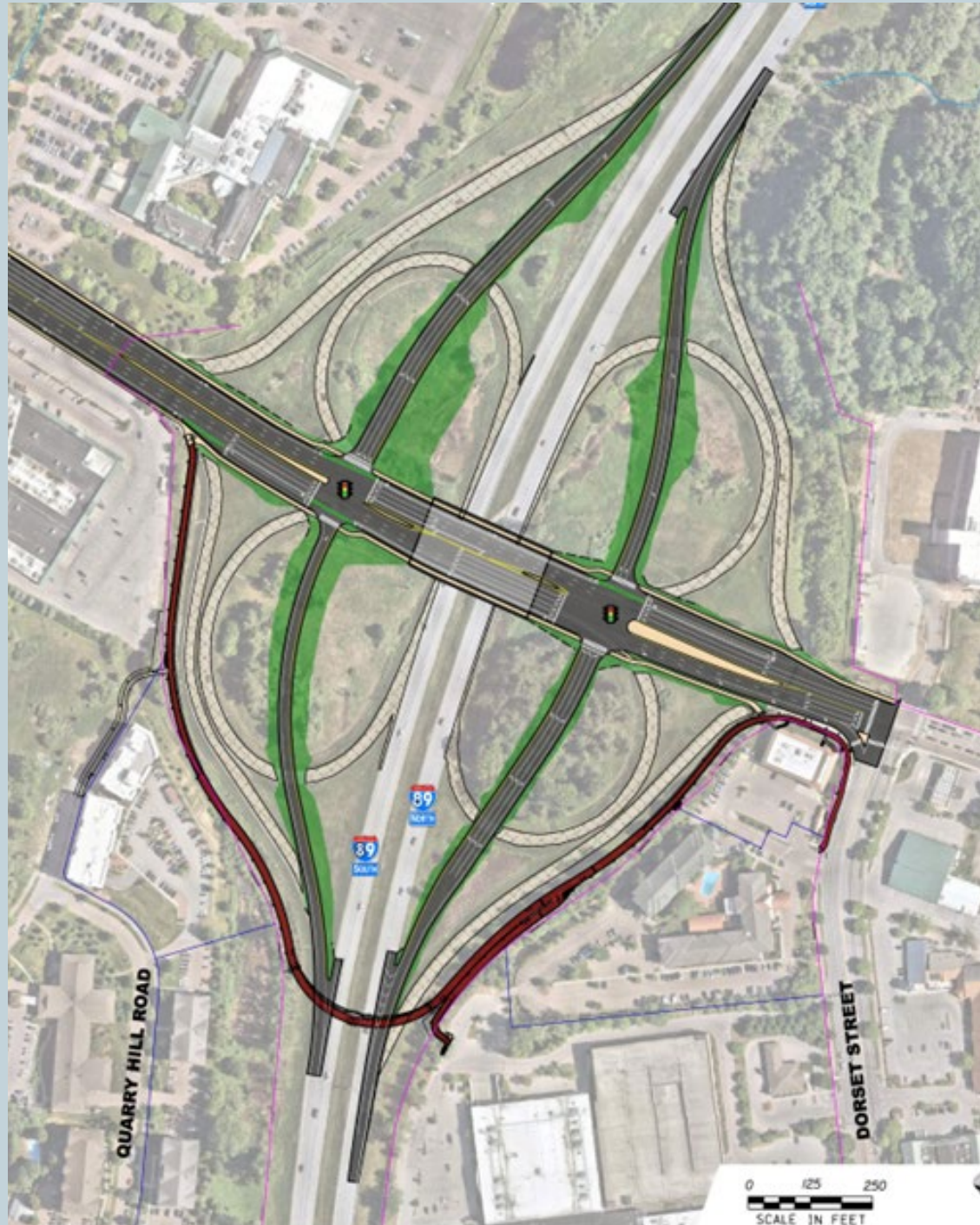
Compressed Diamond Interchange
