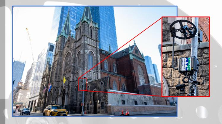
Following the New York City pilot refinements were made to the system which included provision of ANPR/ LPR cameras, a wide angle/ vehicle tracking camera and a microphone array which is used to detect the dominant noisy vehicle (even when there are multiple vehicles in the imagery).
