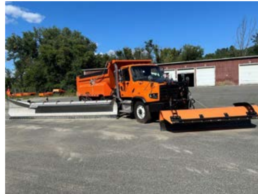
The Agency has purchased a Megaplow named “The Vermonster” to plow I-89. This 21’ plow can plow both lanes at the same time.
