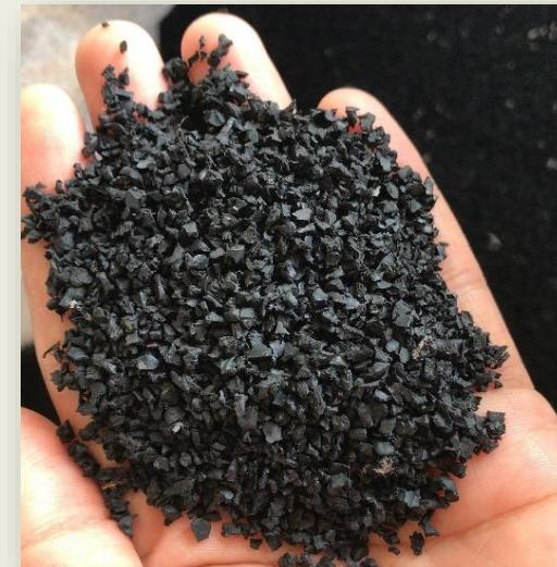
Large Truck Tires processed into crumb rubber. CR sold to rubber flooring manufacturers, molded rubber products manufacturers, dairy cow mattress manufacturers, artificial turf installers, etc.
