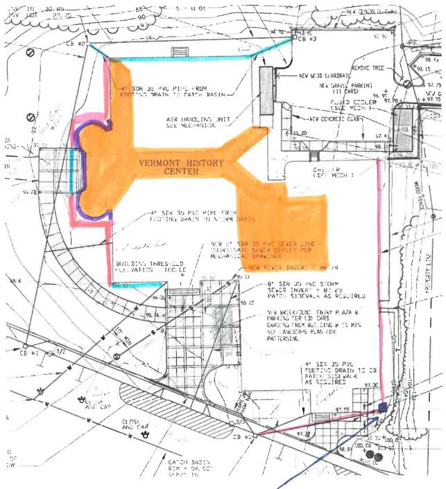
The existing shallow catch basin would be upgraded to a deeper precast structure and tied into the new foundation drain piping and tied into the city stormwater system at catch basin #5, by replacing the damaged pipe connecting the existing catch basin to CB #5.
