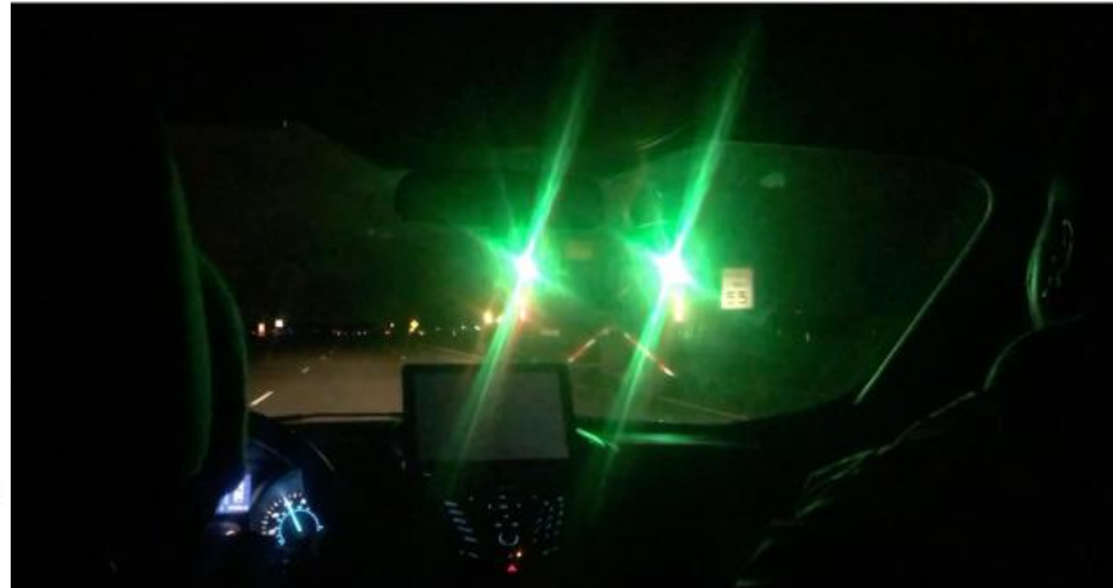
Figure 4-9 Conspicuity, appropriate driving action and glare rating tests in the dynamic experiment
