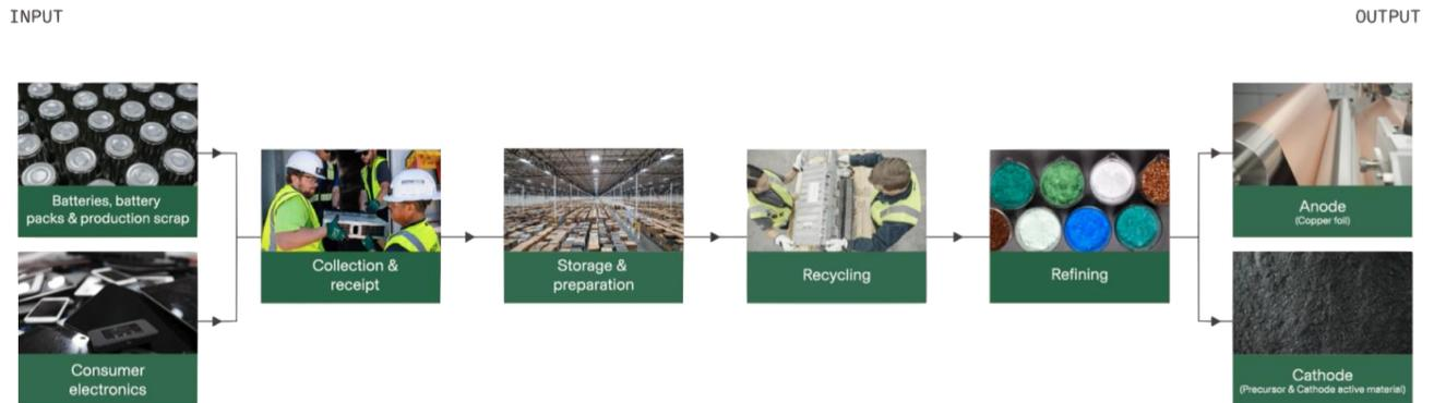
Figure 5.1.4.1: Example of the Redwood Materials Recycling Process.<sup>231</sup>
