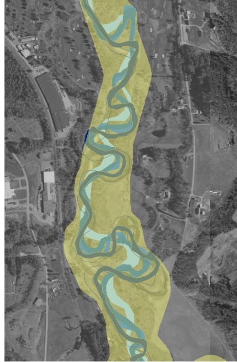
Figure 8: Limiting new encroachments along undeveloped river corridors allows for rivers to maintain or restore a least erosive condition and maximize natural and beneficial floodplain functions, including the storage of floodwater and sediment.
