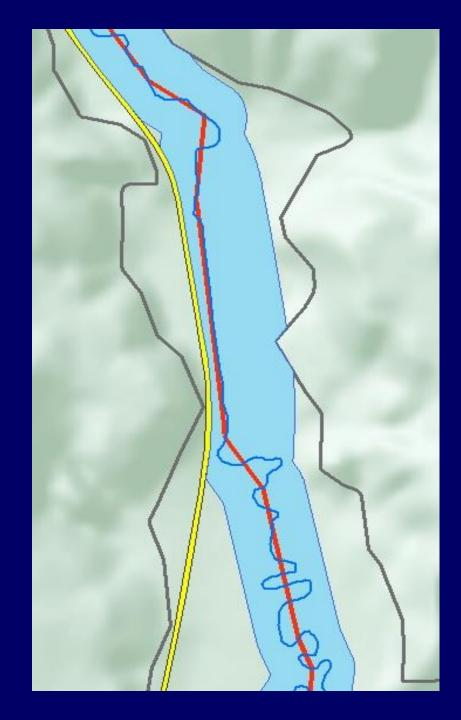
Meander Belt Width-based corridors are designed to accommodate the slope and pattern of the equilibrium channel at the end of the evolution process. Used to support river corridor planning and protection.
