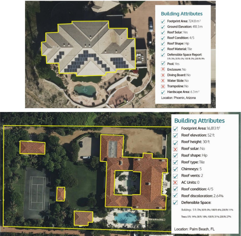
Figure 15: Summarized Building Attributes. In examples from Arizona and Florida, the presence or absence of property features and measurements are quickly assessed and provided.
