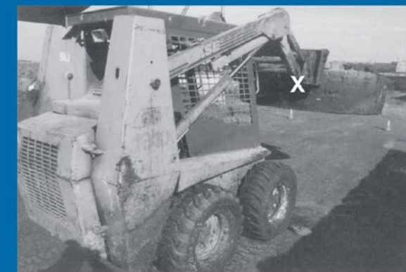
Photo 1: A 23-year-old Hispanic laborer died after being crushed between the frame of a skid steer loader and the scraper attachment on the loader lift arms at a rendering plant. The manual and warning signs at the site were available in English only.
