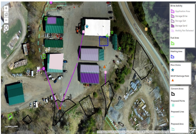
FIGURE 1. Annotated map of stormwater-related areas of concern/action at the AOT St. Johnsbury Maintenance Facility
