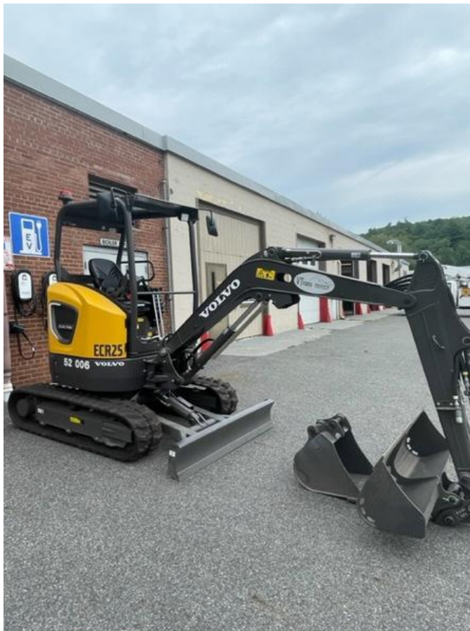
The battery powered all-electric ECR25 Compact Excavator is the first model in a new line from Volvo, making it the first electric machine of its kind in our fleet. This piece of equipment produces zero emissions and less noise, reduces energy costs, and requires less maintenance.
