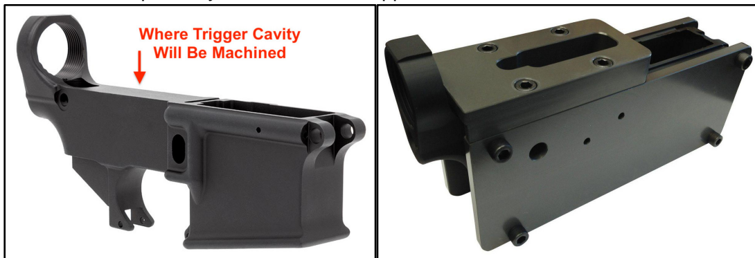
An “80-percent” lower receiver for an AR-15 on its own (left) and placed in a jig (right).
