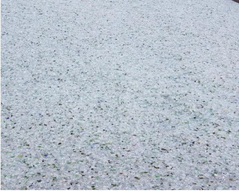
Picture of Clear Recycled Glass (Flint) – Furnace Ready. – this is end market product with stable positive market price.
