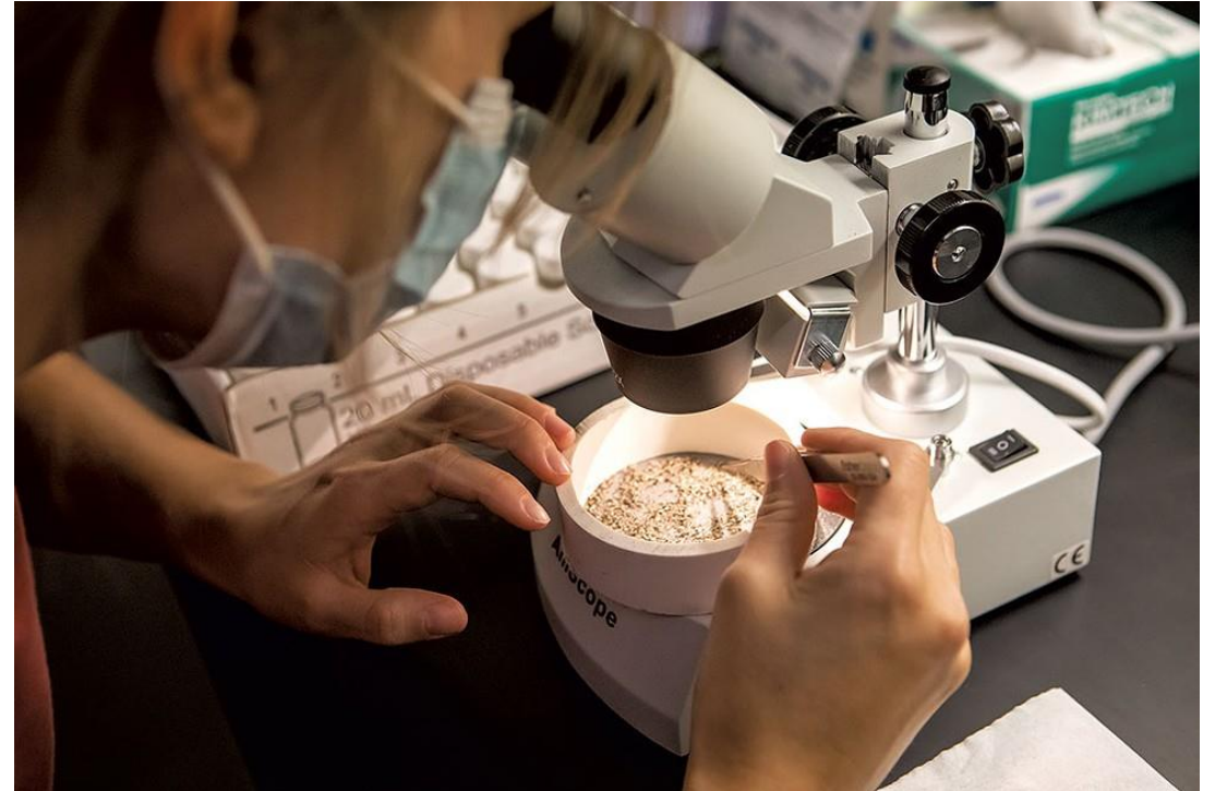
Kate Porterfield a PhD student of Civil and Env. Engineering at UVM examines sieved particles for microplastics. Photo credit: Luke Awtry Photography.
