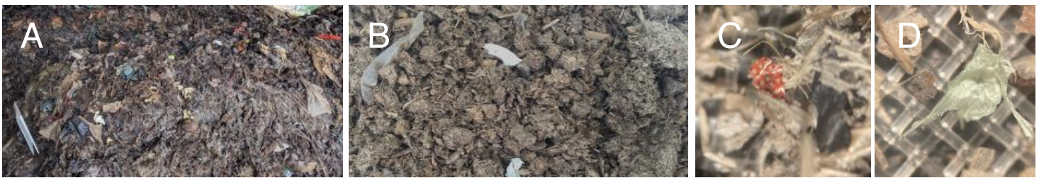
Figure 2. Visible plastic contamination in (A) organic municipal solid waste compost windrows prior to screening (credit: E.D. Roy, S. Asia), (B) screw-press separated solid digestate from co-digestion of dairy manure and food waste (credit: E.D. Roy, United States), and (C–D) Putative microplastics found in food waste digestate (credit: K.K. Porterfield, United States).
