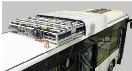
Above: an AKASOL lithium-ion battery for electric buses. Image: greencarcongress.com . Below: cross-section of a battery mounted on the roof of an electric bus. Image: 100percentelectricbuses.wordpress.com .
