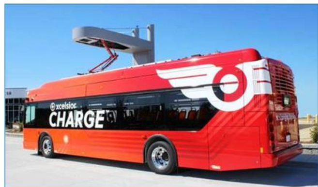
A New Flyer electric bus gets an in-route charge from a pantograph-down overhead conductive charger. This type of charger allows for charging of a bus at a layover or other location away from the depot at speeds faster than most plug-in chargers and do not require a maintenance crew member to perform the operation.
