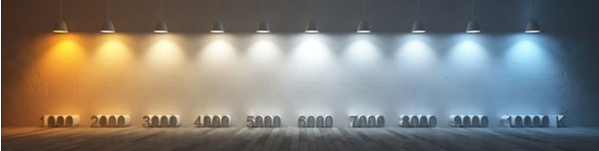
Figure 5. Picture of different CCT Light Colors and their Corresponding CCT value in Kelvin
