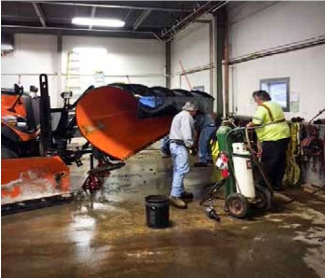
Maintenance workers replace a plow blade in preparation for a coming winter storm.
