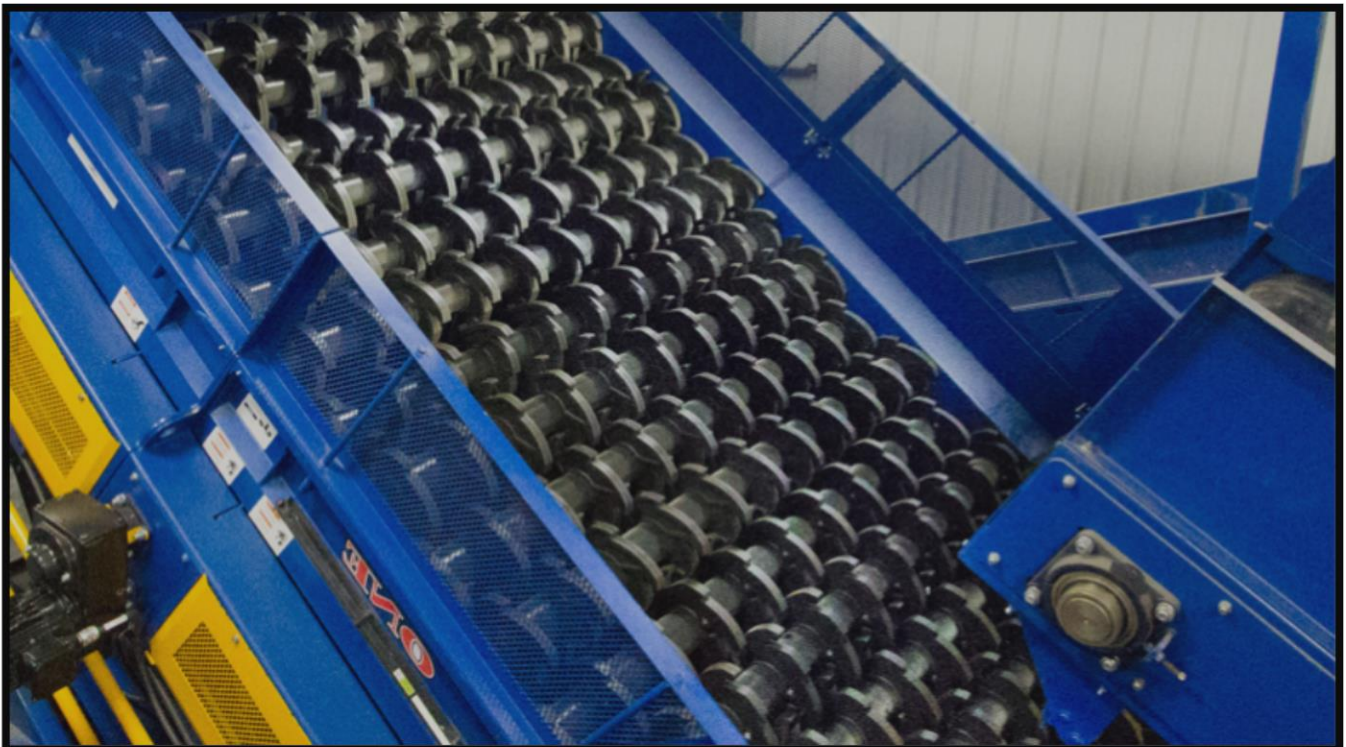
MRF star screens when new, as they are intended to function.
