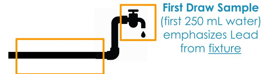
Flush Sample (water collected after 30 sec flush) emphasizes Lead from <u>pipes</u>
