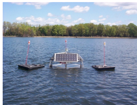
SolarBee Circulator installed in Lake Champlain, St. Albans
