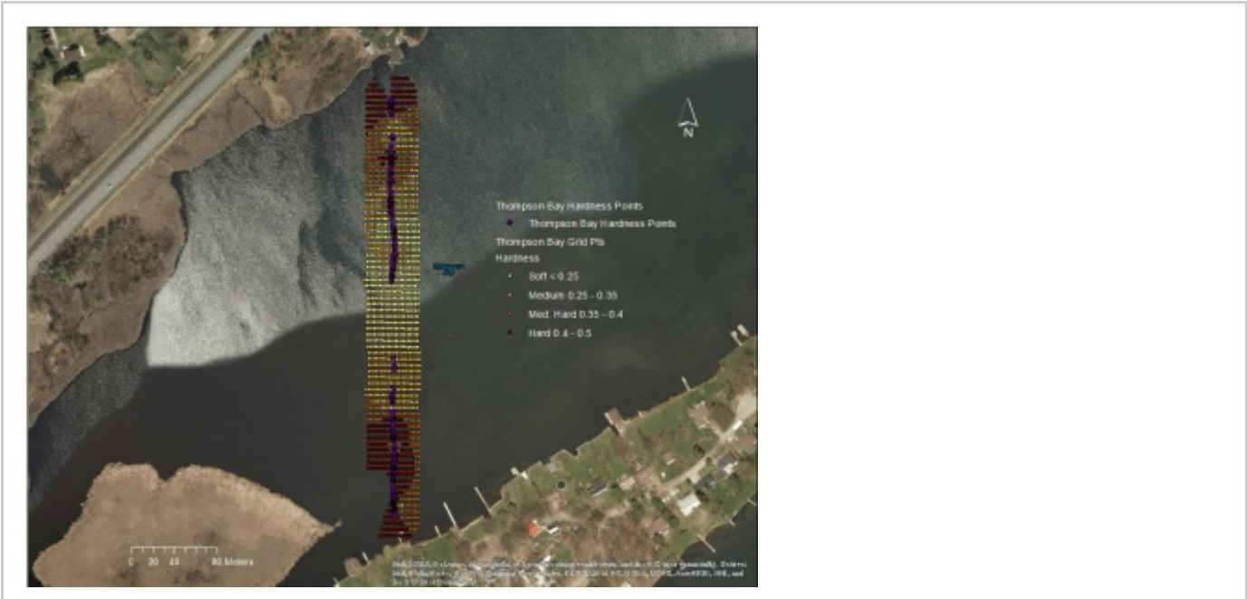
Figure 6. Example of kriging hardness grid points overlain with coordinate points exported from EcoSound and added to ArcGIS as a text event layer (WGS84 coordinate system). Kriging data values outside of the transects (extrapolated) may not be accurate. However, the map directly over the point values should be accurate. In this example, it is recommended that the user only use the point hardness data and not the grid data.
