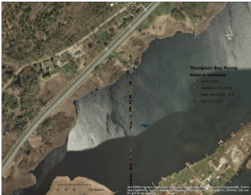
Figure 4. Bottom hardness point data exported from EcoSound and imported into ArcGIS. The different colors indicate the bottom hardness scores. Notice the large gap in the data where vegetation was the most dense (see Figures 1 and 5).
