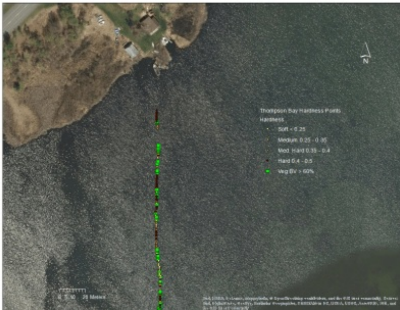
Figure 5. Bottom hardness point data overlain with vegetation point data > 60%. Notice the lack of overlap of data anywhere where dense vegetation occurred and hard scores where it didn't occur.
