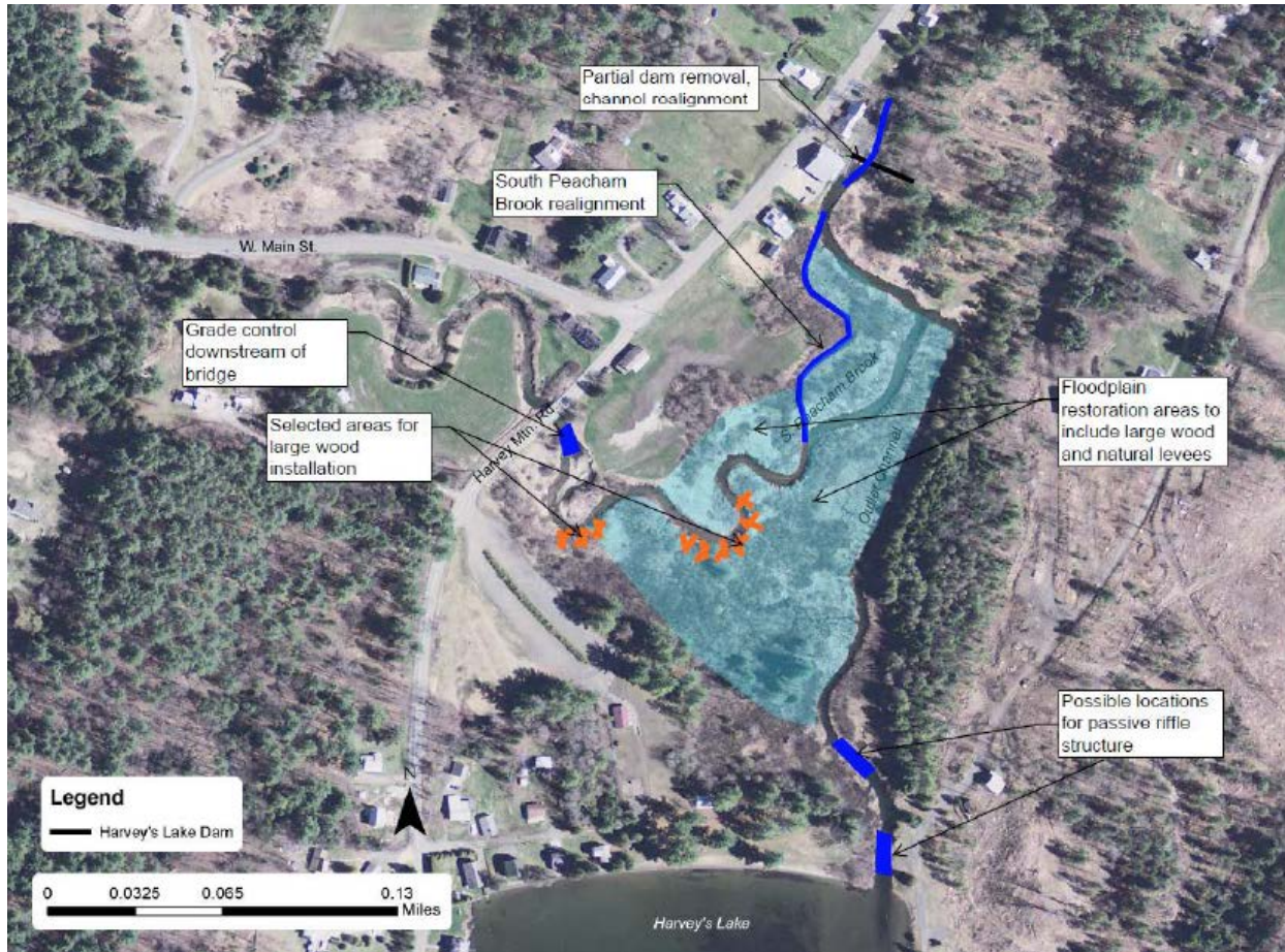
Figure 26. Preliminary design concept for Harveys Lake Dam removal (2018 Harveys Lake Design Concepts Report, Interfluve).
