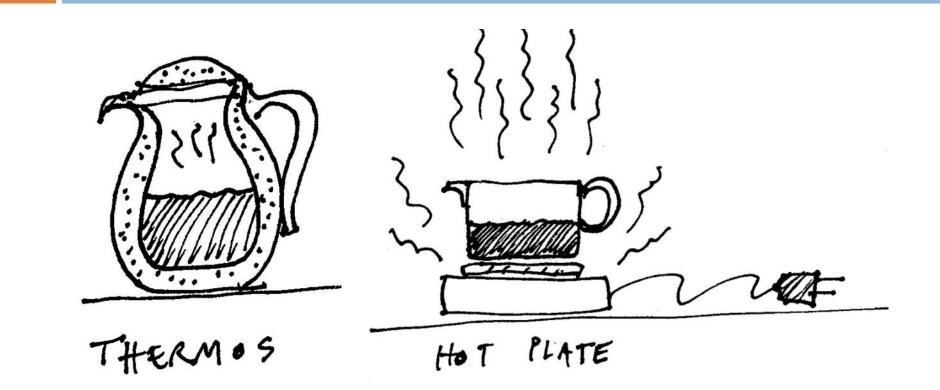
Maintain the temperature using insulation, rather than by using energy.
