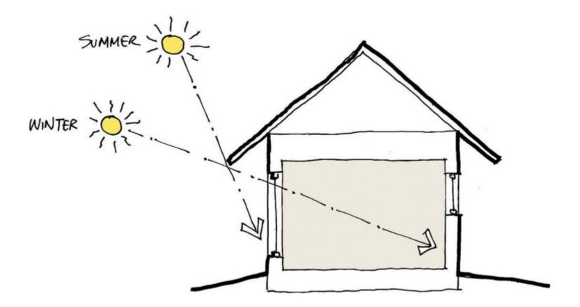
TRIPLE GLAZED: U VALUE < 0.13; 0.60 Solar Heat Gain Coefficient on South Windows for Climate Zone 6
