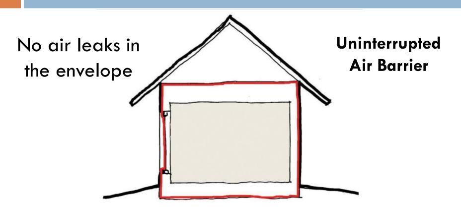
Max. 0.6 ACH @ 50 PA ( based on interior floor area) Max. 0.05 cfm/gross sqft shell @ 50 PA Blower Door Test limits
