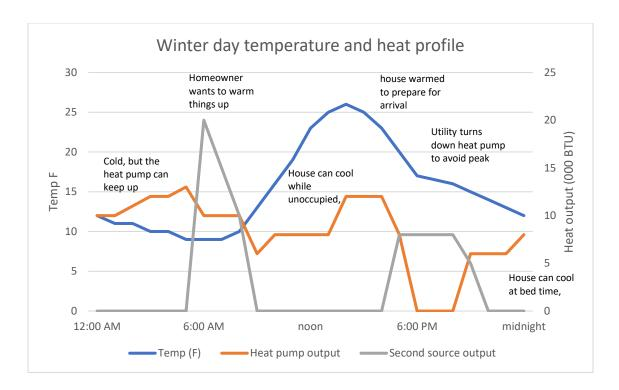
Note that using a heat pump without proper controls; the electricity demand will peak during the morning and early evening – the times that the electric grid is in highest demand.
