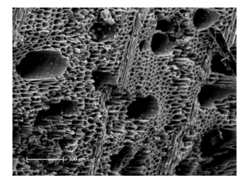
Hardwood Biochar at high magnification. The pits and tubes are hollow. One nanometer is one meter divided into one billion parts. The scale at lower left shows the length of 100 nanometers, or one part in 100 million.
