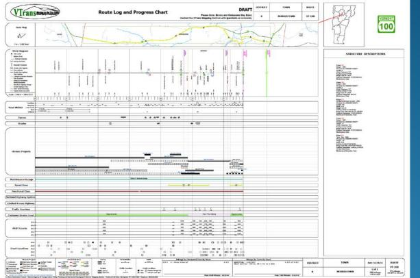
The Section produces approximately 1600 Route Logs, which are straight line diagrams of the federal aid highway system, providing detail on geometrics, projects, AADT, crashes and other pertinent information.
