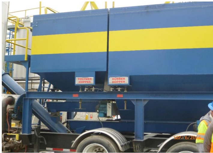
Portable hot mix asphalt plant, Hooksett, NH, incorporating ground tire rubber.
