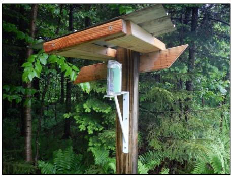
Photograph 5. Time-lapse camera mounted adjacent to LS-A9. Shed roof was added to prevent rainwater from obscuring lens during storm events (VHB, 06/05/2016)
