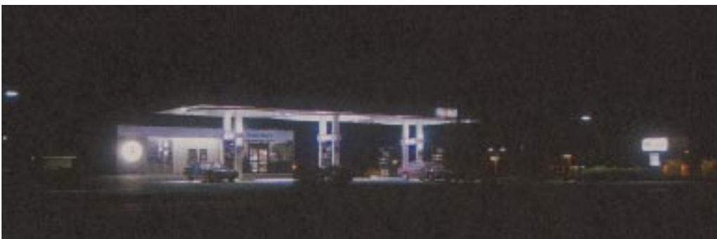
Gas stations should be visible but not overlit. Appropriate lighting such as this, focuses light in the pumping area and doorways where it is needed. Source: Outdoor Lighting Manual for Vermont Municipalities.
