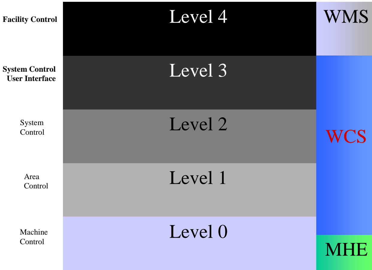
Figure 0.12 - Conceptual control system architecture
