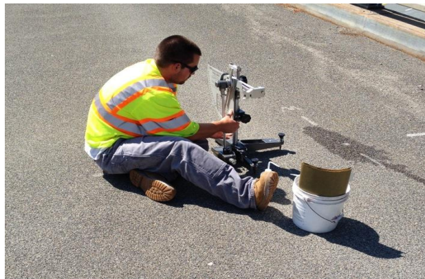
British Pendulum Testing on a Friction Surface Overlay
