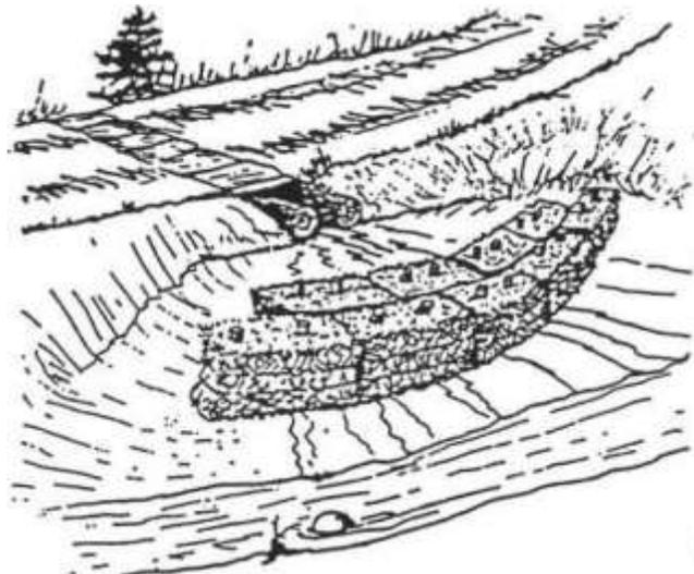
figure 7: Haybale Erosion Check.
