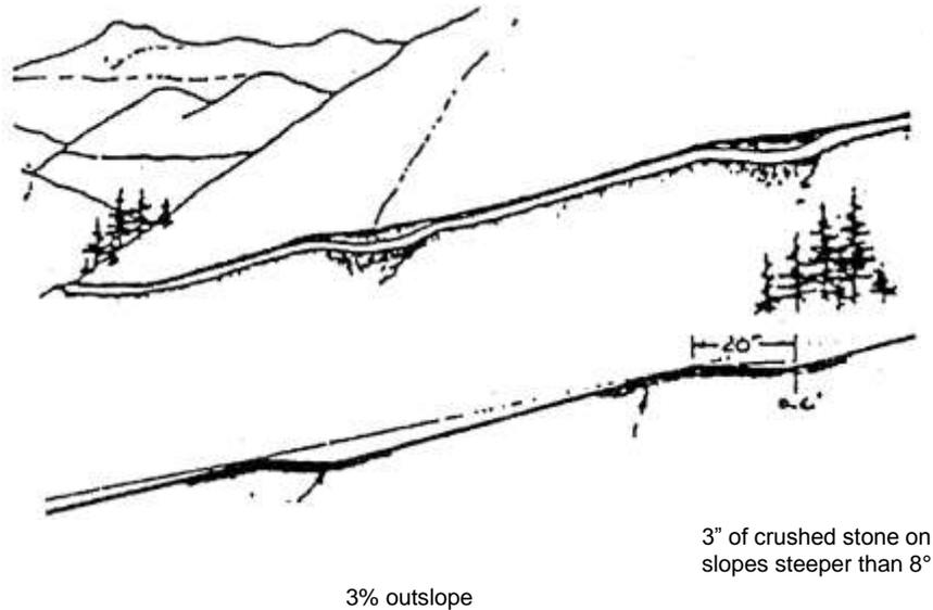
Figure 3: Diagram and Design of Broad-Based Dips on a Mountain Logging Road.
