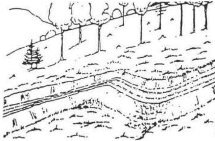
Figure 6: Turnups. Cross drainage can be obtained by turning the skid trail up the hill a few feet then turning downhill again.
