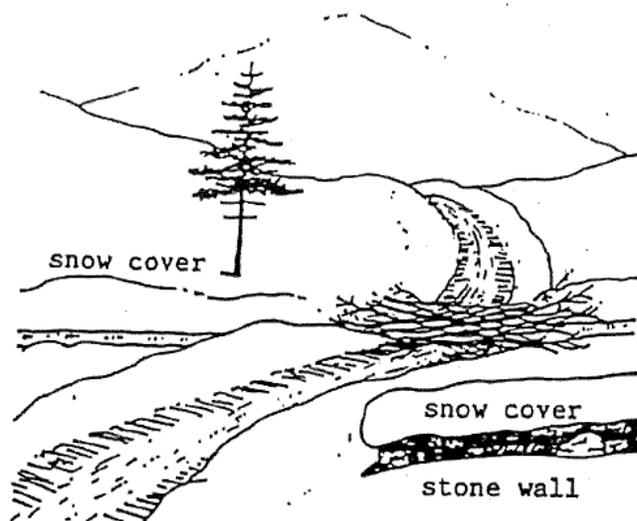
Figure 10: “Brushing-In” a Streambed. During Frozen Winter Conditions.
