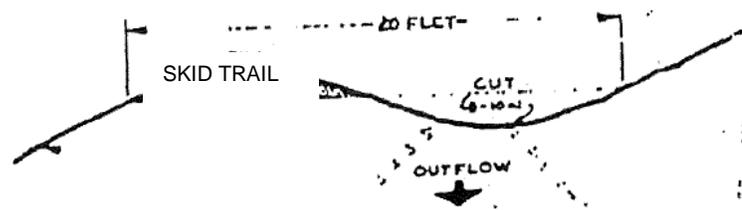
Figure 4: Specifications for the Construction of Standard Drainage Dips Used During Logging.
