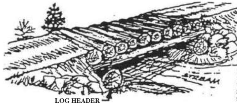
Figure 8: Design of Simple Header Bridge.
