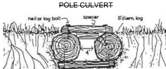
Figure 2: Proper Construction of Pole Culverts on Logging Roads.
