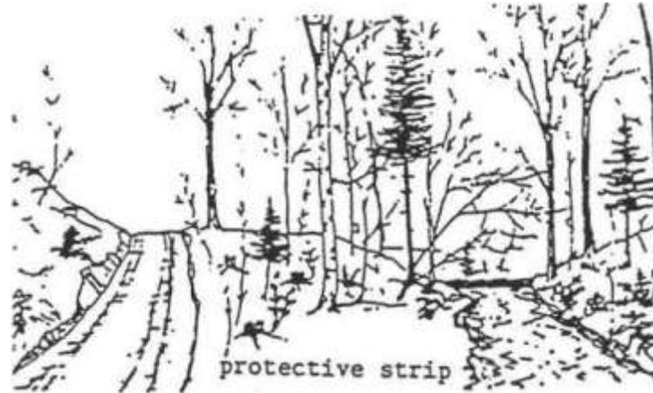
Figure 11. Protective Strip. A protective strip prevents sediment from reaching streams and maintains shade and streambank stability.
