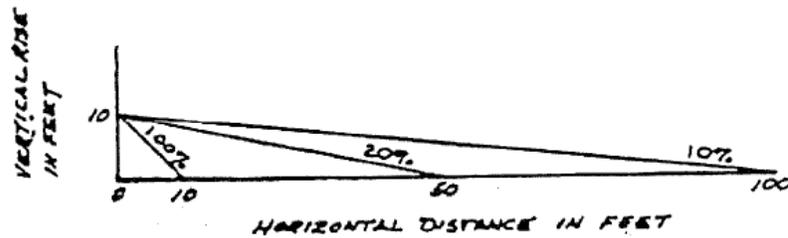
~~Figure 1: Slope Percent. Slope percent is calculated by dividing the rise or elevation by the run or horizontal distance. For example, a slope that gains 10 feet of elevation over 100 feet of horizontal distance is a 10 percent slope:  $10 \div 100 = 10\%$ .~~
