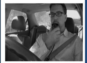
A camera eliminates the excuse that the interlock violation was by another person. It also ensures the offender is the one using the device. The camera is safely mounted near the dashboard.
