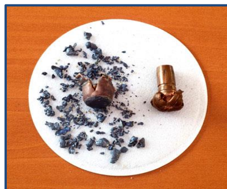
Two different .270 caliber bullets show how lead (left) disintegrates when it penetrates while non-lead (right) expands and mushrooms upon impact. (© National Park Service)
