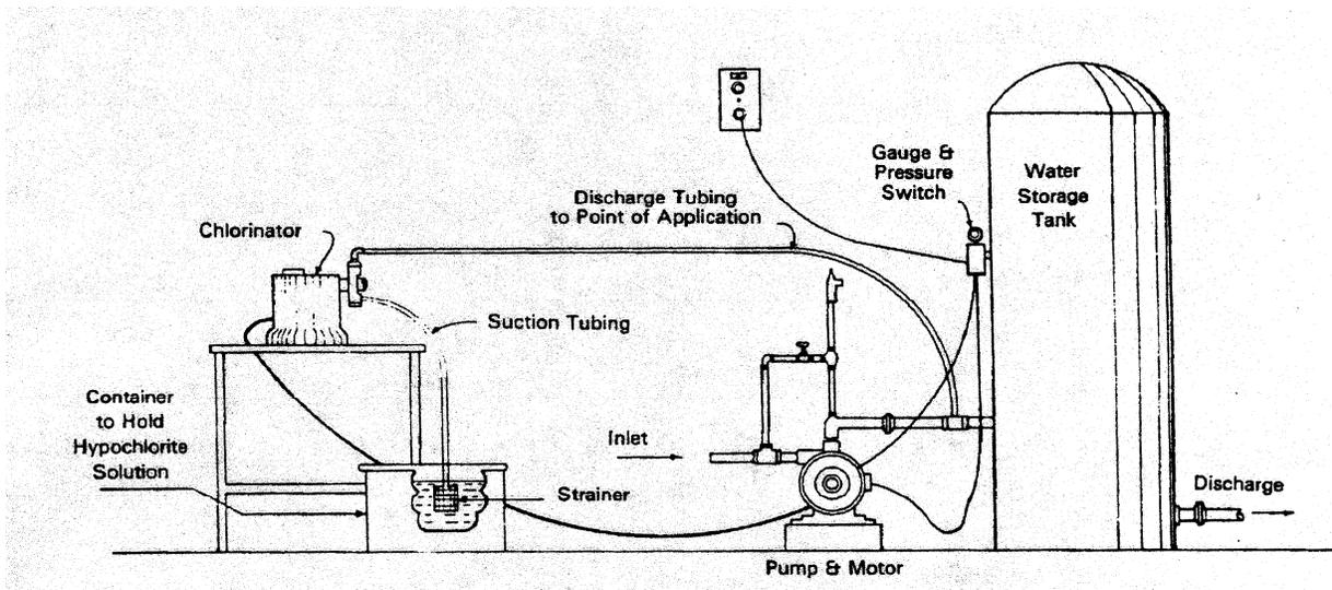
Figure 30. Positive Displacement Chlorinator
