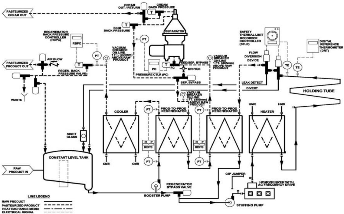
**Figure 35. HTST Pasteurizer with a Booster Pump, Homogenizer as a Timing Pump with an AC Variable Frequency Drive, CIP-Type Separator Located Between Two Pasteurized Product Regenerators and an Air Actuated Discharge Valve with an Air Blow**
