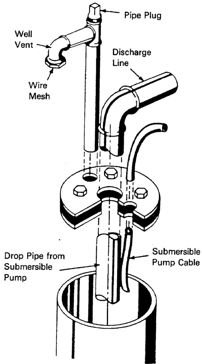
**Figure 27. Well Seal for Submersible Pump Installation**
