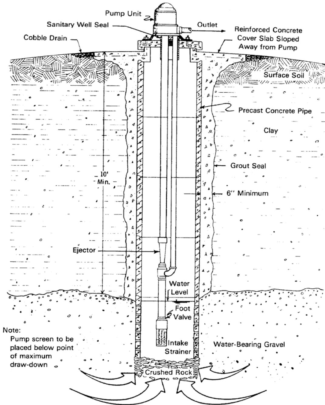
**Figure 15. Dug Well with Two-Pipe Jet Pump Installation**
