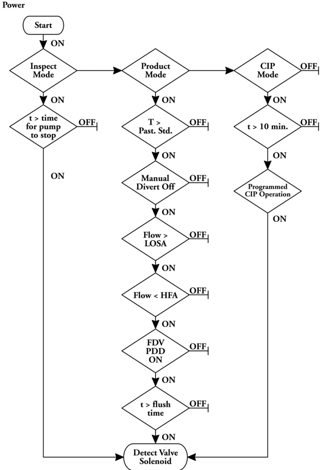
Figure 53. Logic Diagram: HTST Flow-Diversion, Leak-Detect Valve Stem
