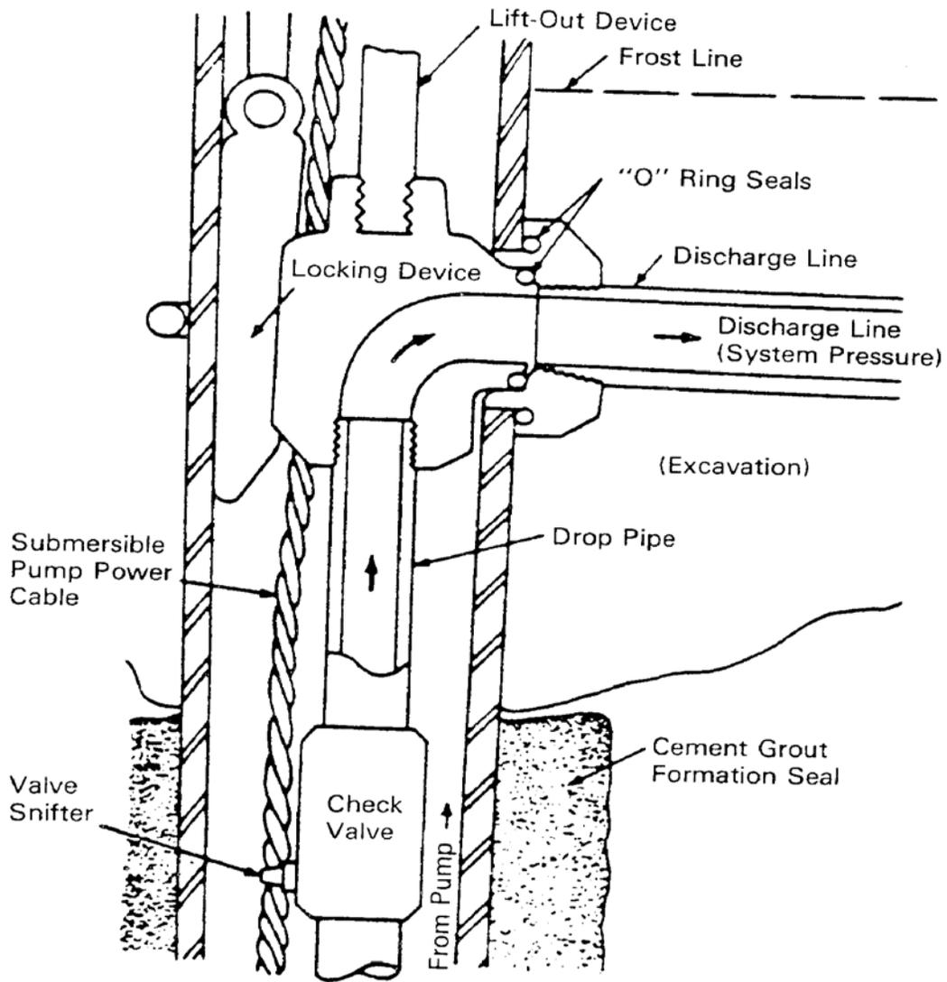
**Figure 23. Clamp-on Pit-less Adapter with Concentric External Piping for "Shallow Well" Pump Installation**
