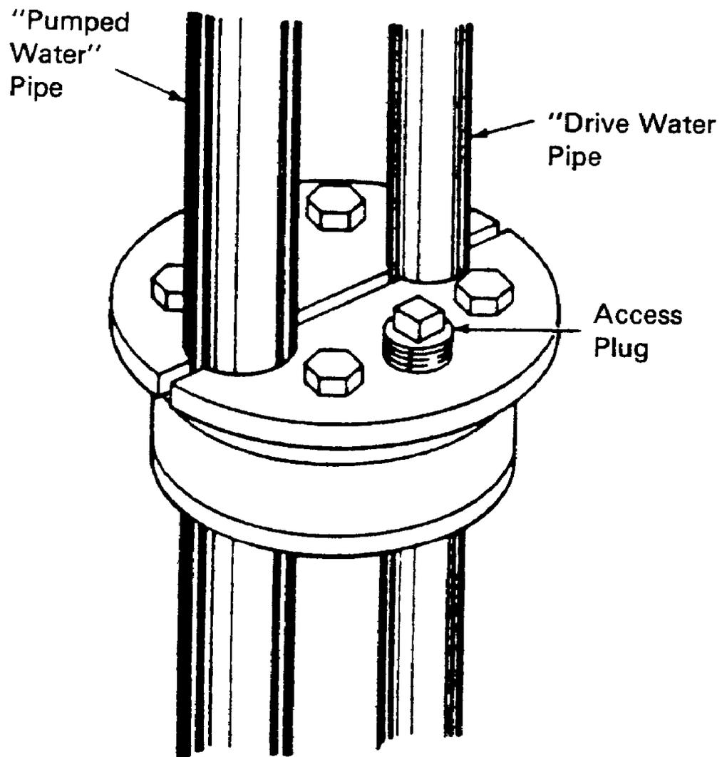
Figure 26. Well Seal for Jet Pump Installation
