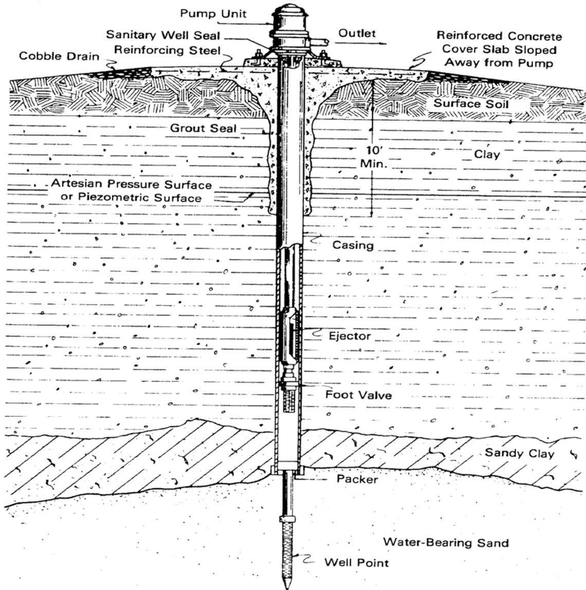
Figure 13. Bored Well with Driven Well Point
