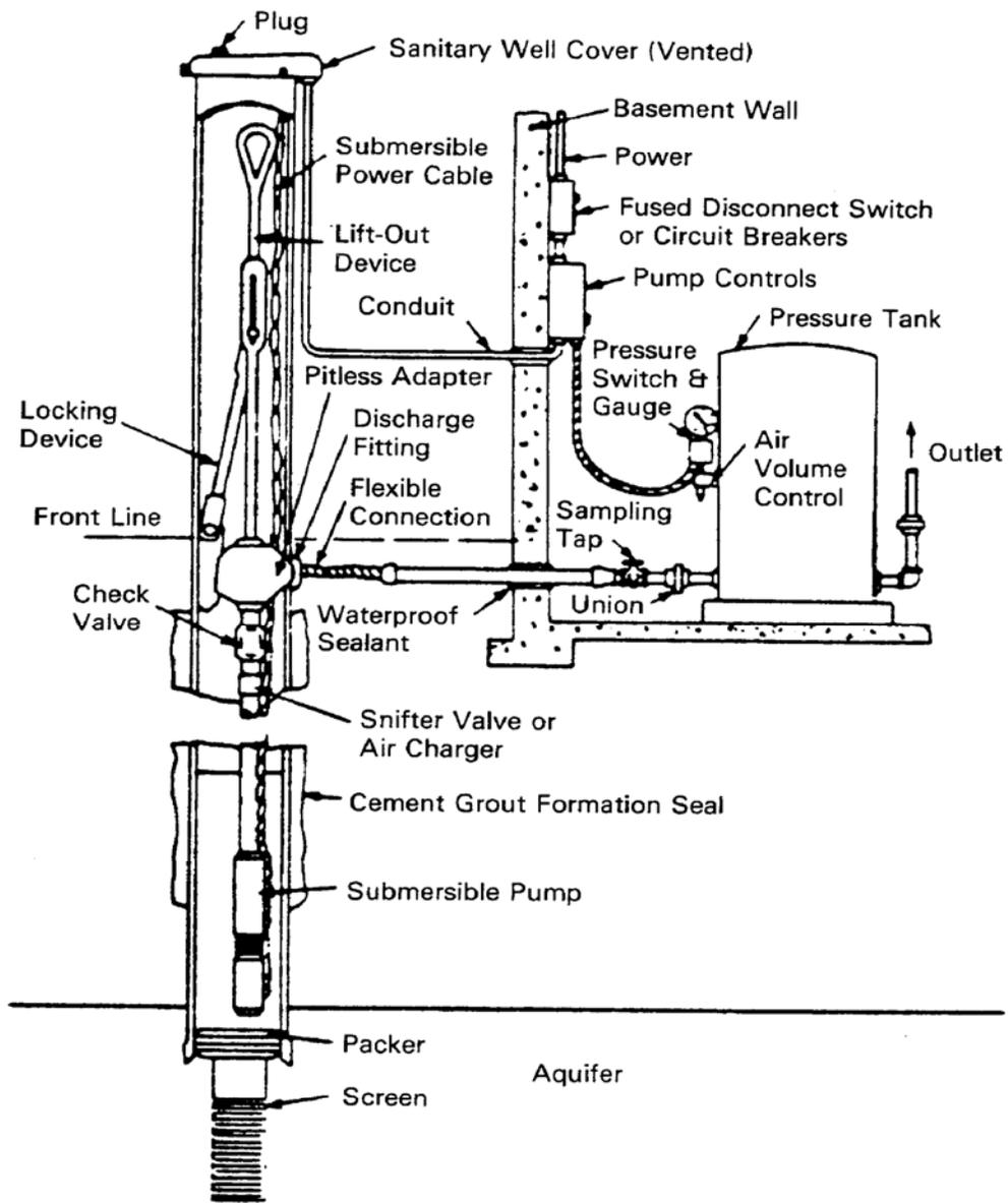
Figure 22. Pit-less Adapter with Submersible Pump Installation for Basement Storage
