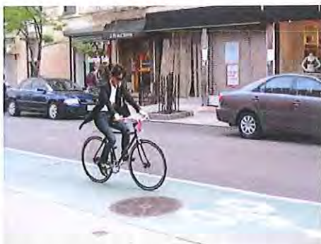
On-street bike lanes are cost effective and relatively easy to instal.This green bike lane is made with paint and thermoplastic pavement markings on an existing Right of Way.
