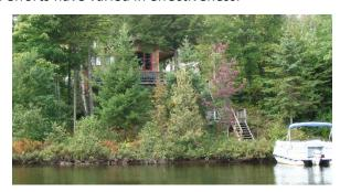
**Figure 3. Lake-friendly shoreland development** includes: setting a lawn back from the lake; allowing native trees to stabilize the bank, while pruning lower branches for a view; leaving woodlands (duff layer, shrubs, and mature trees) in place to filter runoff and provide healthy habitat for fish and other wildlife.
