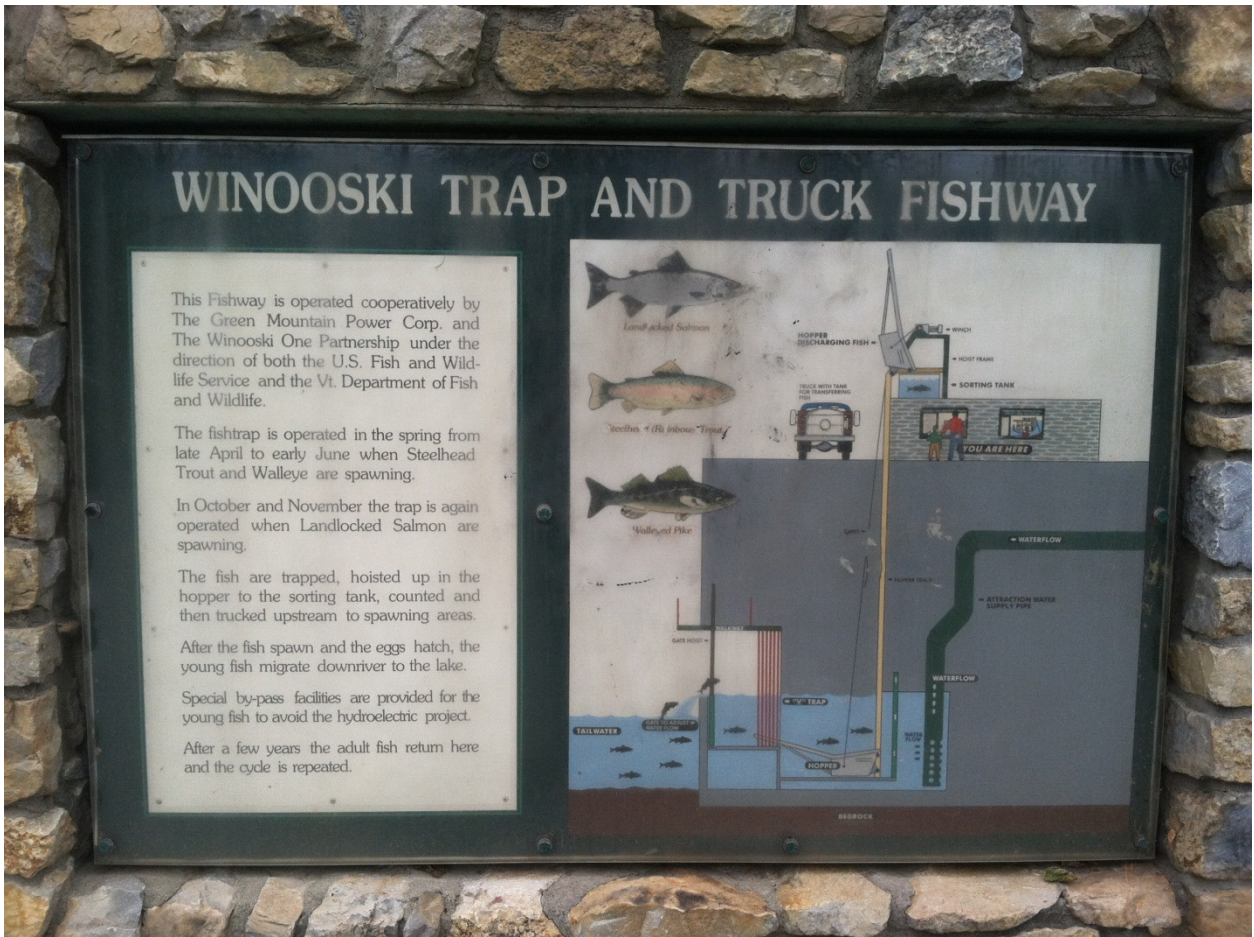
Figure 13: Winooski One Fish Lift. Diagram of Winooski One Dam outlining fish lift, an ecological mitigation strategy
